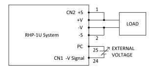
+S & +V, -S & -V also need to be connected on CN1. (Only for power supply system)
